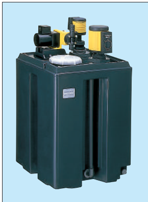
■Best choice for implementing "full" alarms on chemical turbid water tanks in waster water treatment and other processes. This is the best choice for corrosive chemicals as it is made entirely of resin. ※We also have a range of tank mixers.
